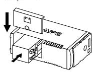
d. Push the battery into the battery compartment and re-install the cover, as shown.
